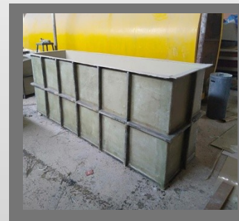
Fabricated PP FRP Tank
